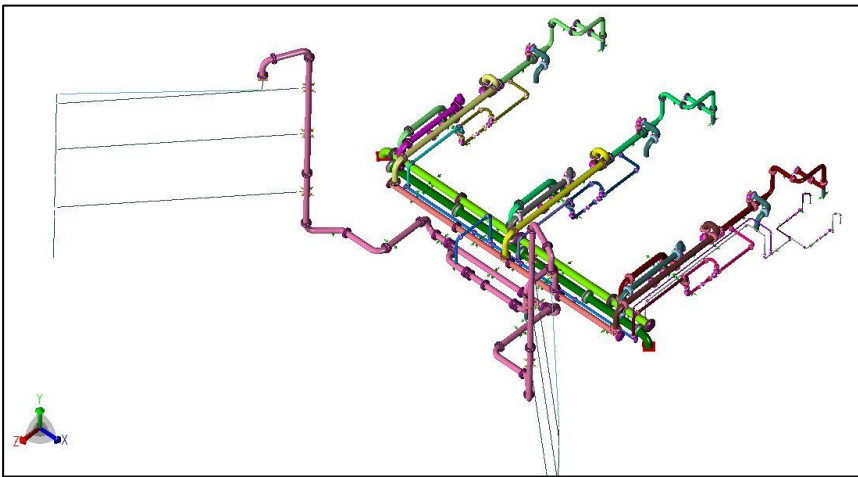
Piping from Pumps to Tanks
