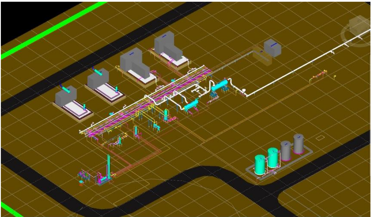
Piping 3D Modeling of Compressor Station
